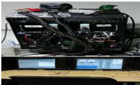
Figure 2 : Physical Hardware in loop set up
