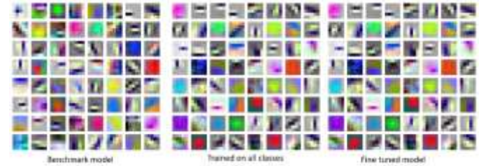
Figure 4.2.1: The images are a representation of the kernels (weights) in the first layer of our trained models. Left most images is the visualization of weights in the first layer of our benchmark model.
