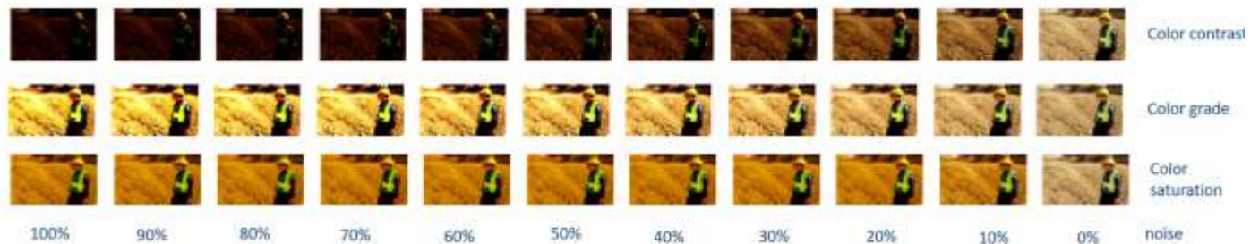
Figure 3 Systematic color variations in the image: color contrast, color grade and color saturation
