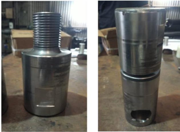
Figure 4: Re-used Machine Part from Inventory as Frugal Load Cell
