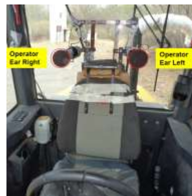
Figure 1. In-cab noise measurement microphone set-up.
