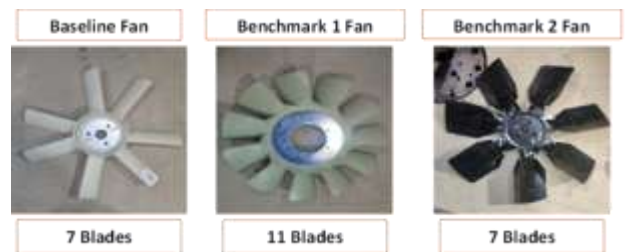
Figure 5. Geometry of different fans used for comparison.
