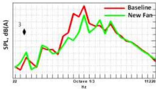
Figure 11. Noise comparison between baseline fan & new fan.
