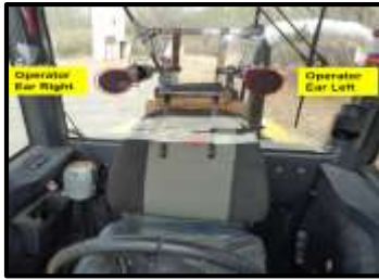
Figure 1. In-cab noise measurement microphone set-up. (Std 6396)
