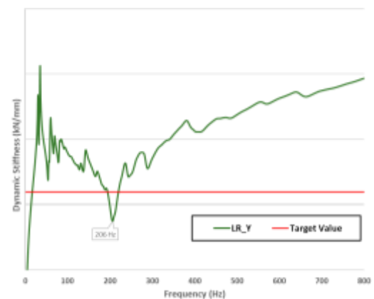
Figure 6: Dynamic stiffness results at LR in Z- Direction
