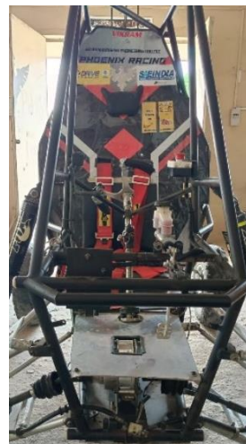
Fig.54. Mounting of Kill switches on the vehicle
