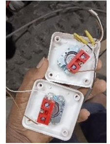
Fig.52. Kill switch – Original image and Opened view of two connected Kill switches
