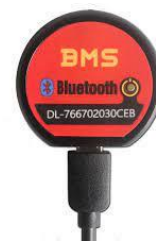
Fig.13. Daly BMS tag used for transmitting BMS data to mobile phone using Bluetooth
