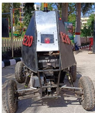
Fig.51. Reverse light and reverse alarm, Their mounted positions on the vehicle
