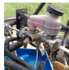
Fig.49. Brake circuit, Brake light circuit and pressure switch
