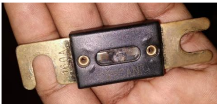
Fig.81. Blown fuse after heavy load application
