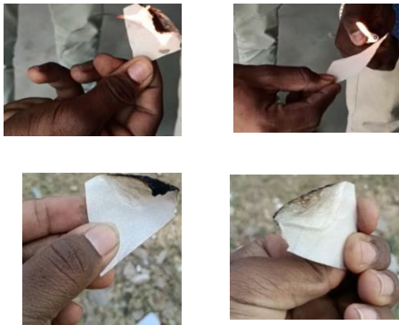
Fig.58. H class Nomex material and flame testing
