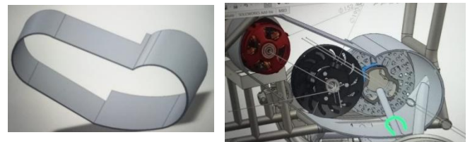
Fig.72. CAD of CVT casing
