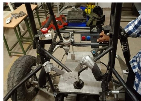
Fig.44. Mounting of driver display in the vehicle
