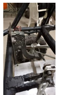
Fig.69. Limit switch and placing of limit switch behind the accelerator pedal
