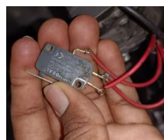
Fig.69. Limit switch and placing of limit switch behind the accelerator pedal
