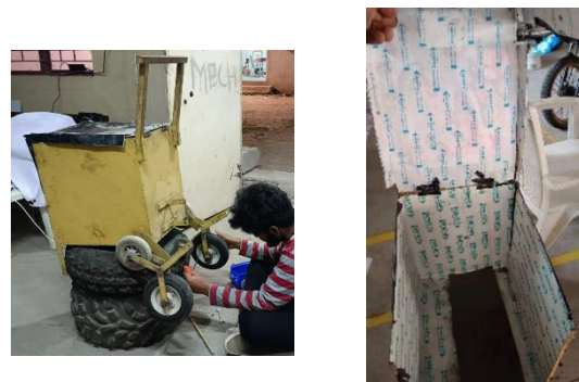
Fig.87. Hand cart fabrication and Insulation coating using Nomex “H” class material
