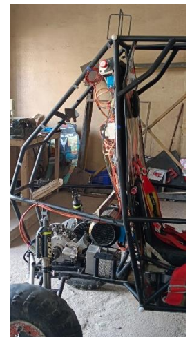
Fig.54. Mounting of Kill switches on the vehicle
