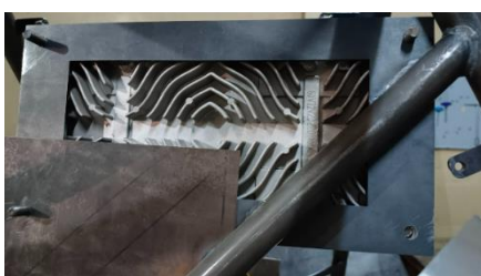
Fig.76. Motor Controller fixing – heat sink with ventilation
