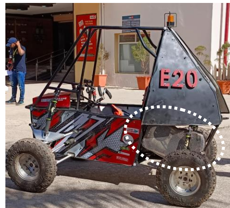
Fig.73. CVT casing with wire mesh – implementation
