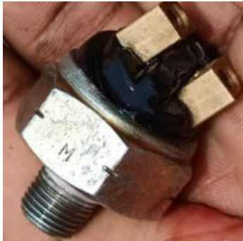
Fig.80. Deformed pressure switch
