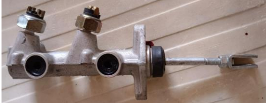
Fig.50. Arrangement of pressure switches on the master cylinder
