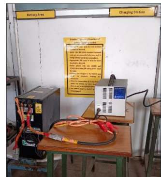
Fig.16. Battery charging setup at garage
