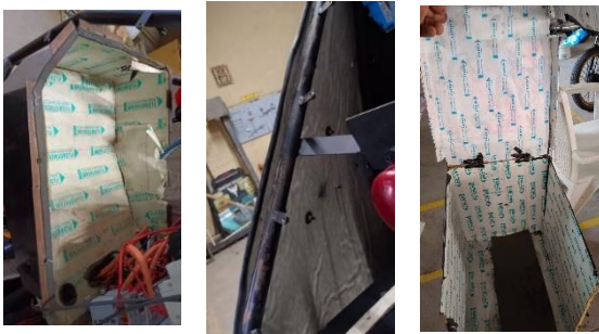
Fig.58. H class Nomex material and flame testing
