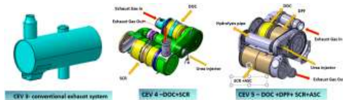
Figure 2: Off highway Exhaust After Treatment System evolution
