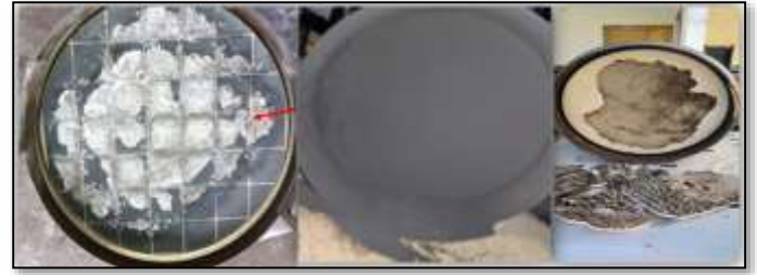
Figure 8: DPF field issues a) DPF clogged b) soot accumulation c)DPF crack or damage
