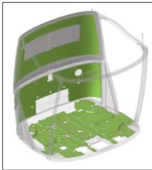
Figure 1: Acoustic treatments used on a typical Off Highway cab.
