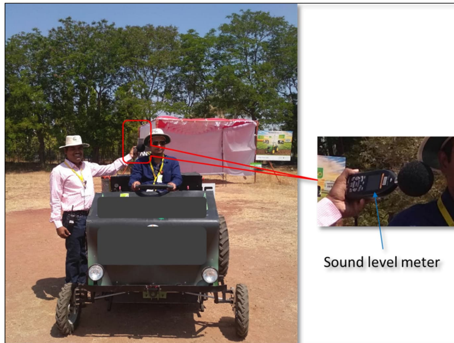
Figure 11: Representation of Operator Ear Noise (OEN) measurement using sound level meter
