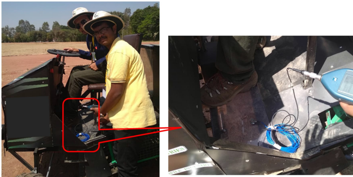
Fig 15. Vibration level measurement at footrest location using vibration meter for self-propelled (Actual Pictures)
