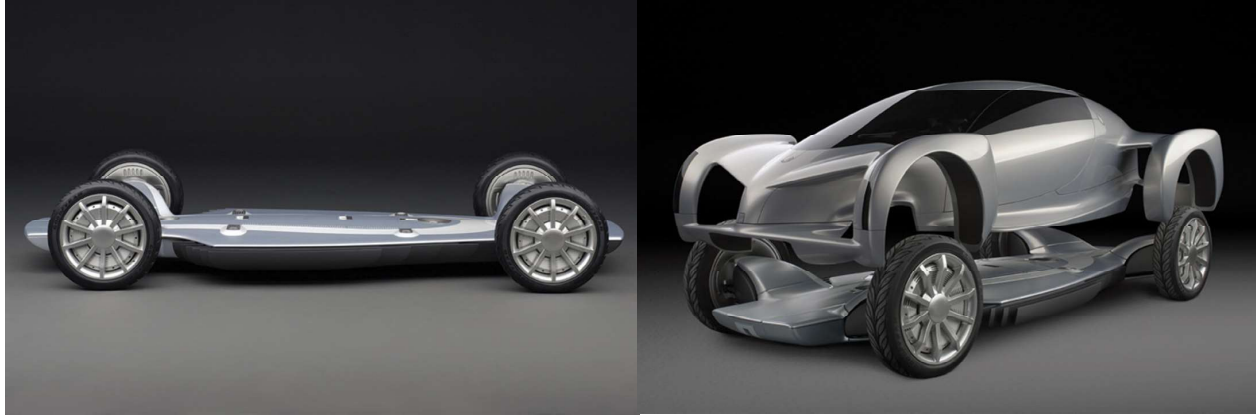
Fig 1. EV AUTONomy Skateboard from General Motors (Ref. [1])
