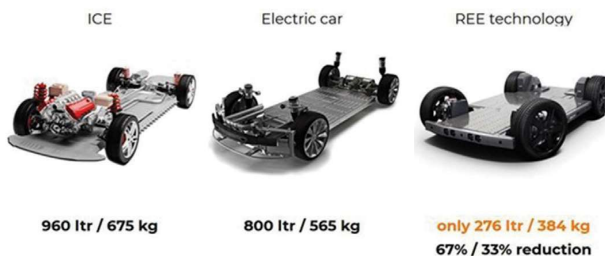
Fig 2. Weight Reduction from ICE to Electric Vehicle to Flat Skateboard with WCM (Ref. [2])
