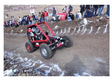
After the Static technical Inspection, vehicles were evaluated for the dynamic events category of maximum acceleration, brake test, slope test and maneuverability, followed by 4 hour durability test on the rough track.
