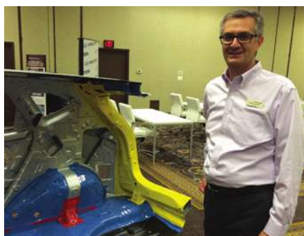
Hyundai's Chahe Apelian next to the Tucson BIW. Note the hot-stamped steel piece (red) that sandwiches the damper, resulting in a 109% increase in rigidity, reduced road noise levels, and ride and handling improvements. (Ryan Gehm)
