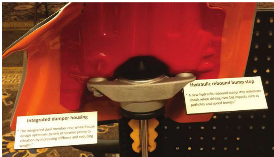
The new Tucson features a "world first" integrated dual-member rear wheelhouse design using AHSS (orange = 100 kg/mm 2 , or 980 MPa; red = hot-stamped steel). Also shown is the hydraulic rebound bump stop. (Ryan Gehm)
