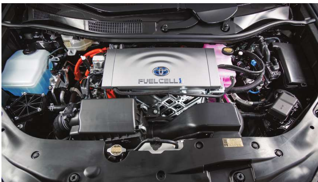
Mirai's fuel cell stack is half the size and 1/20th the cost of the stack that powered Toyota's previous FCV.
