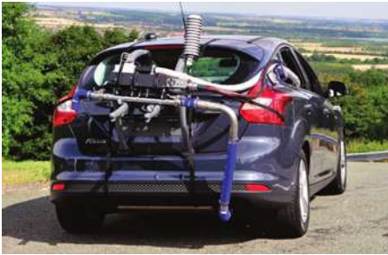
Millbrook has increased its investment in its Portable Emissions Measurement System (PEMS).
