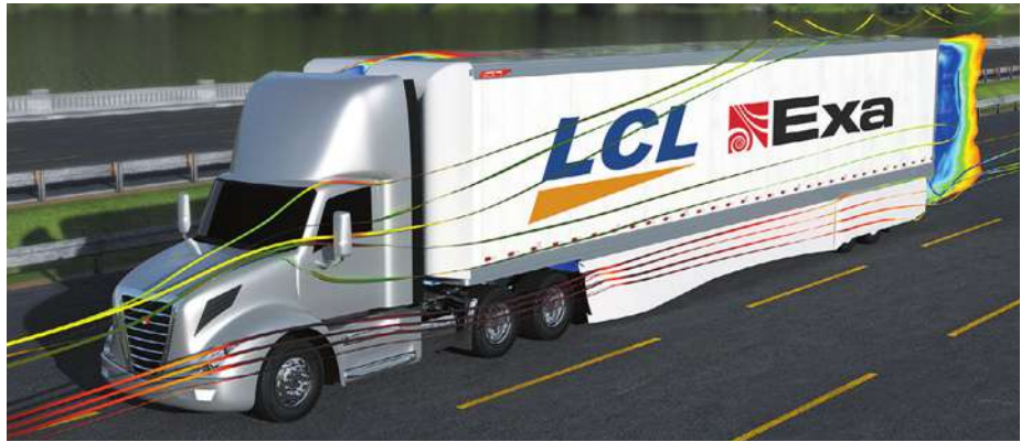
Exa recently worked with Laydon Composites on a trailer skirt solution that explored which design would provide optimum results. The result of extensive simulation was a 9.3% improvement in fuel economy, and achieving U.S. EPA SmartWay Elite status without a boat tail.
