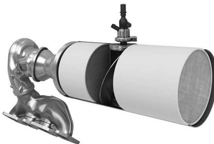
In a cutaway view of the double-swirl mixer, urea injection takes place in the small space between the oxidation catalyst and SDPF.
