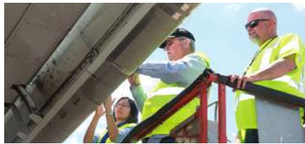
NASA materials scientist Mia Siochi and systems engineer Mike Alexander, from the agency's Langley Research Center in Hampton, VA, and Boeing technician Felix Boyett count insect residue on the right wing of Boeing's ecoDemonstrator 757 aircraft following a flight test in Shreveport, LA. (Credit: NASA Langley/Paul Bagby)
