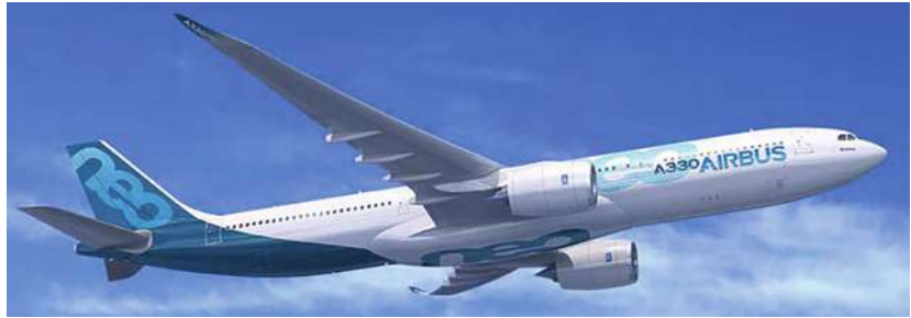
Rolls-Royce's Trent 7000 being developed for application on the upgraded A330neo (shown is the -900) offers better all-round performance than the Trent 700 it replaces.
