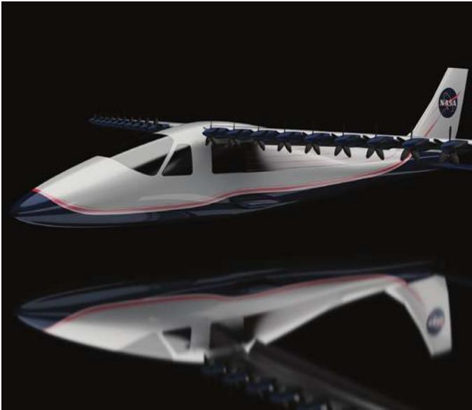
NASA plans to replace the wings and engines of Tecnam light plane with an improved blown wing featuring multiple props.
