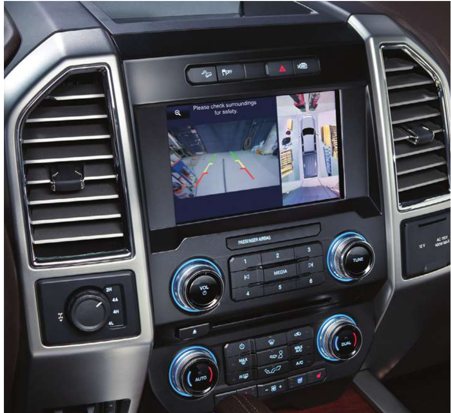
360° camera display screen in the 2015 F-150 pioneers Ford's adoption of this safety technology across its global truck and SUV ranges by 2020.
