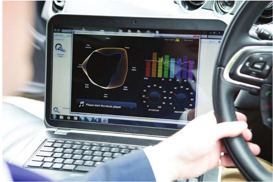
Driver concentration and "wellness" monitoring systems are being developed by JLR.
