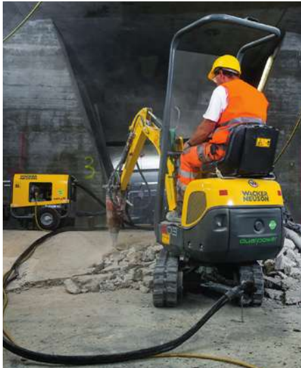
If Wacker Neuson's 803 is required for demolition/renovation work or interior restorations, the operator can drive it in conventional mode to the site of operation. Two openings are embedded in the excavator's dozer blade in which the HPU8 can be suspended for transport.
