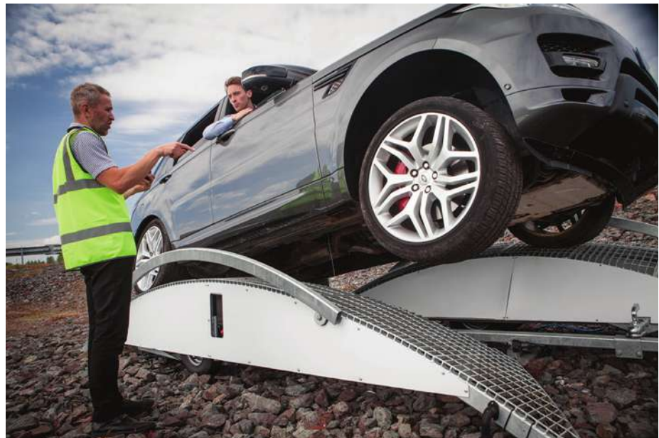
Three wheels on the ground and no driver: JLR's R&D remote control off-road system.
