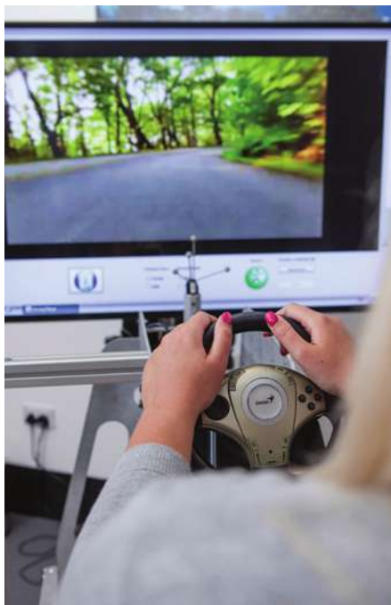
JLR's R&D Mind Sense project, headed by Dr. Laura Millen, monitors driver concentration and alertness via brain waves transmitted from steering wheel sensors.
