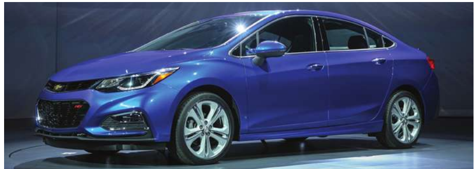
Overall height on the 2016 Cruze has been reduced by nearly an inch versus the 2015 car, which helps enable a 0.29 Cd.
