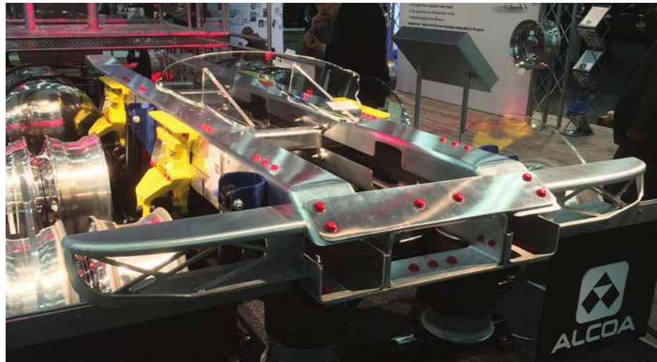
An aluminum truck frame developed by Alcoa and Metalsa, and employed in the SuperTruck program, is 40% lighter than steel frames of the same size. (Images by Ryan Gehm)
