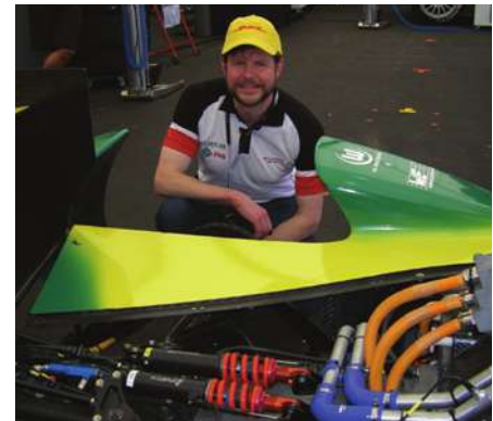
In the paddock area, Schaeffler's Jeff Hemphill looks at an Audi Sport ABT racecar with the electric motor, battery pack, and other electrified powertrain components exposed. All FIA Formula E racecars in the 2014/2015 season have a power output for practice and qualifying of 200 kW. The power output for the race is 150 kW, plus an additional power output of 30 kW by fan voting for three drivers. (Kami Buchholz)
