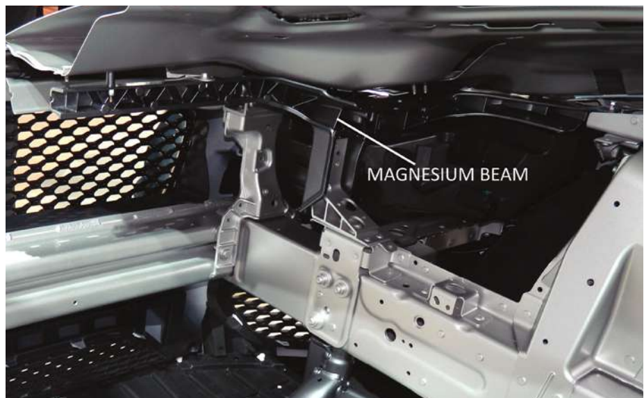
Magnesium is used for XF hood crush beam, as shown, and dashboard cross-car beam.
