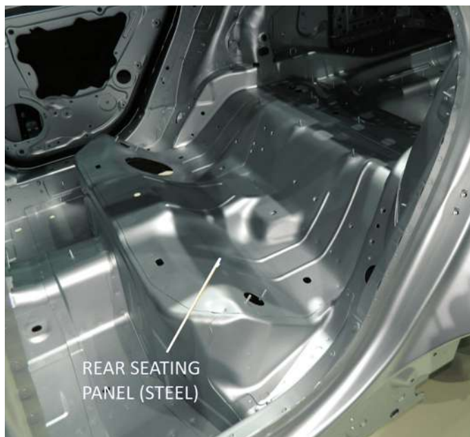
Rear-seat panel is steel, in part for XF weight distribution, and requires multi-step joint to prevent galvanic corrosion with aluminum body.
