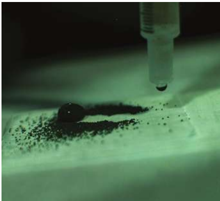
Water beads up on a super-hydrophobic surface, creating spherical droplets that roll along picking up dirt.
