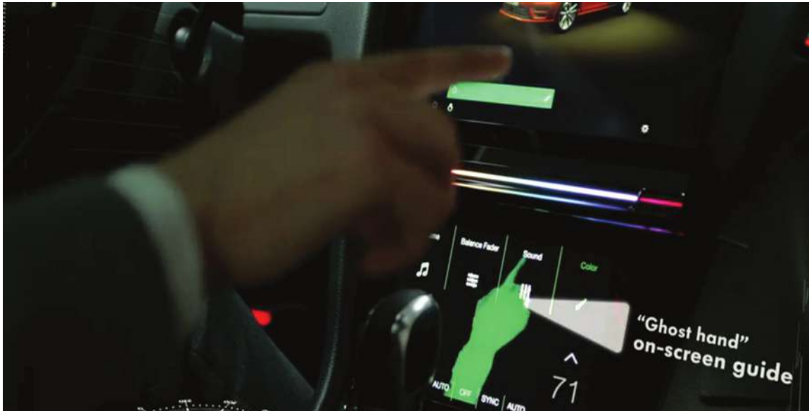
Volkswagen demonstrated that contactless multi-finger gestures can control infotainment in the Golf R Touch at the 2015 Consumer Electronics Show in Las Vegas.
