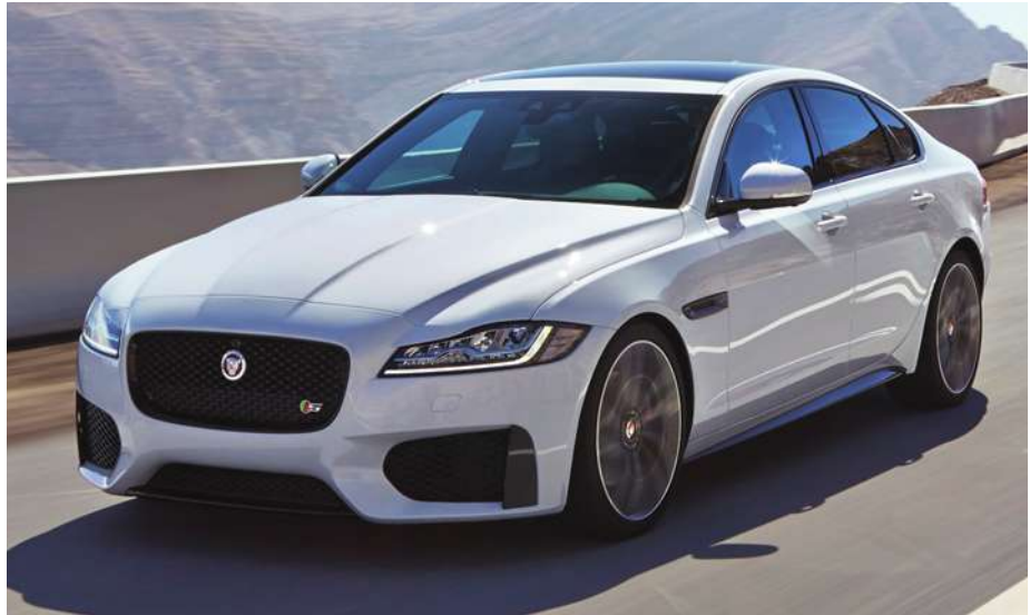
Jaguar XF moves to aluminum body, with a coupe-like look, but with increased rear passenger room, including up to 1.1 in greater headroom.
