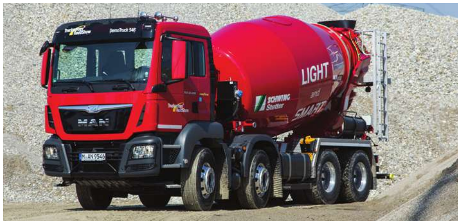
MAN Truck & Bus AG vehicles are built to afford a great deal of versatility. The MAN TGS (shown) can be configured as a two-, three-, or four-axle vehicle and in standard, medium, all-wheel-drive, and ultra-low heights.
