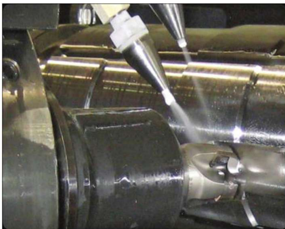
Cooling via CO 2 from an external source.
