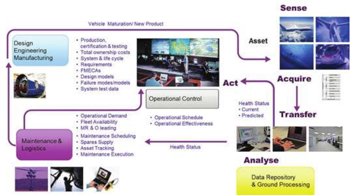
Figure 1. Overview of the main elements of an IVHM system. (IVHM Centre, Cranfield University)
