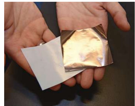
The ultrathin copper sensor is deposited atop a conventional battery separator (white square) as part of an early warning system to alert users that a lithium-ion battery is overheating. (Mark Schwartz, Precourt Institute for Energy, Stanford University)
