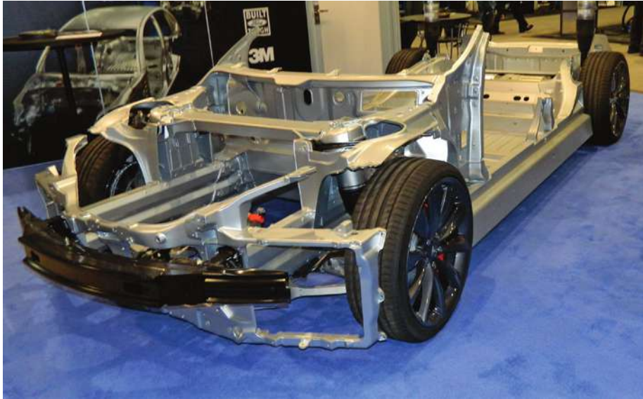
This Tesla chassis is all aluminum, and structural repair parts are restricted to approved shops. It was on display at the SEMA Show by SCRS.
