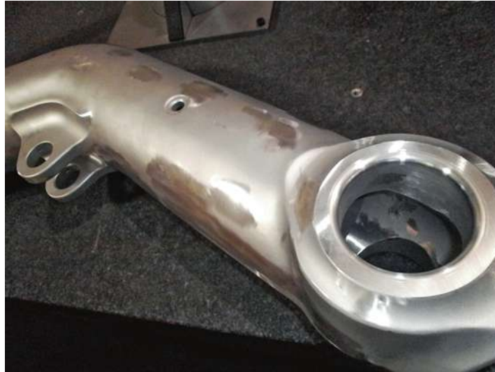
Actual part after removal of corrosion. The shiny areas where it was sanded are clearly visible.
