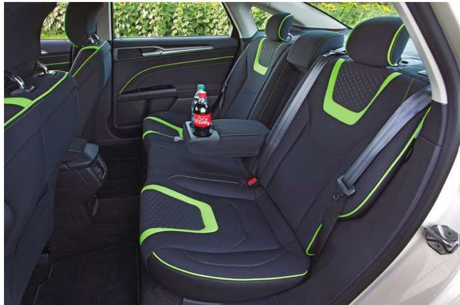
A Ford Fusion Energy plug-in hybrid research vehicle’s interior fabric, containing up to 30% plant-based material, is made from The Coca-Cola Company’s PlantBottle Technology (trademarked). The car’s PlantTechnology is used for seating upholstery, door panel inserts, headliner, and carpet mats. The renewable-fabric research car debuted at the 2013 Los Angeles Auto Show.
