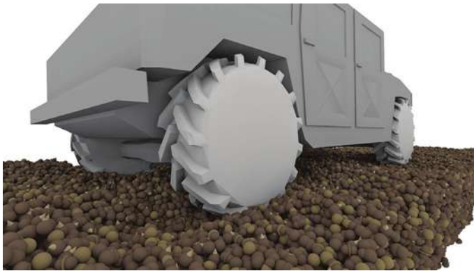
The muddy terrain simulation consisted of a 3000-kg (6600-lb) HMMWV and four rigid 60-kg (130-lb) wheels with treads. A bed of 200,000 objects of varying shape were created with a density of 1250 kg/m 3 .
