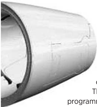
Coriolis Composites and SAFRAN Aircelle worked together on the component, an inner fixed structure (IFS) made of two monolithic carbon skins and a core (above).
