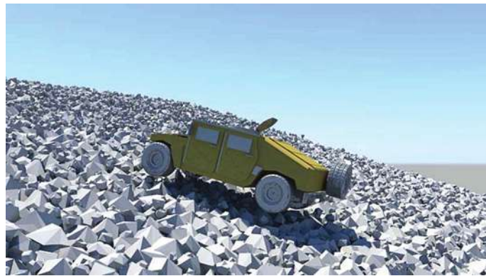
A rocky slope was modeled in Chrono to represent a common obstacle that military vehicles face in gravel hill operations. The terrain's slope varies from 14° to 20° and is composed of over 8000 unique rocks with a randomly generated polyhedral collision geometry.
