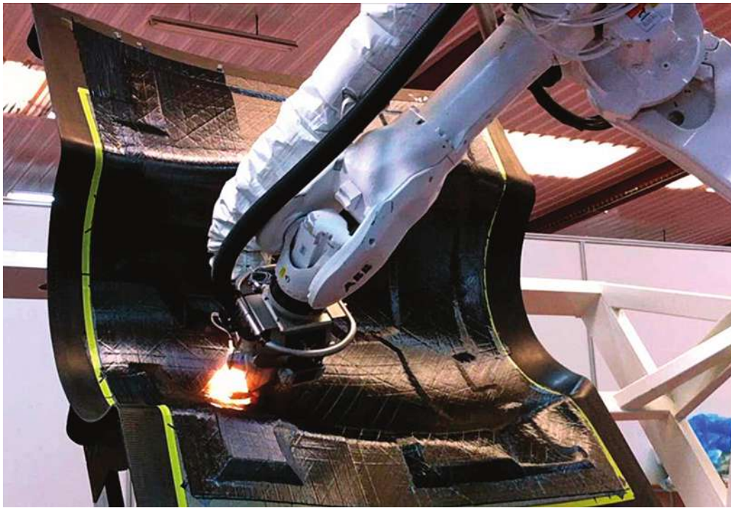
Final layup of cover skin of IFS demonstrator using the Coriolis Composites AFP robot.
