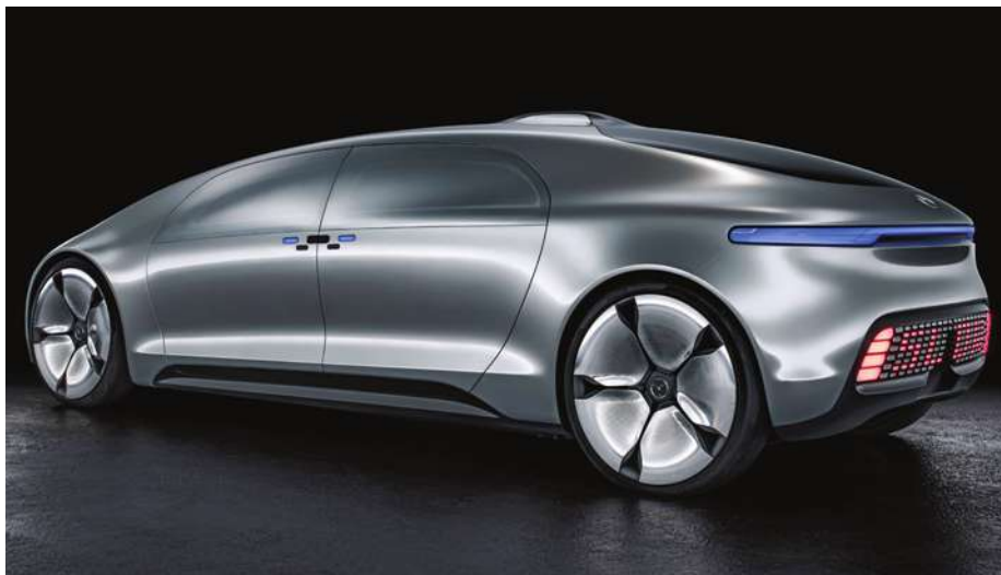
The F 015 has large communication displays at the front and rear with LED panels. By changing the color of the lights, the vehicle indicates what driving mode it is currently in: blue for autonomous and white for manual.
