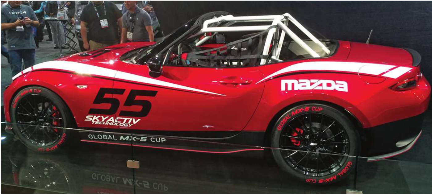
The Global MX-5 Cup racecar will be equipped with a 2.0-L SkyActiv-G four-cylinder engine. Mazda Motorsports plans to undertake a development period this winter to select the optimum tires, suspension, powertrain, and safety modifications. (Ryan Gehm)
