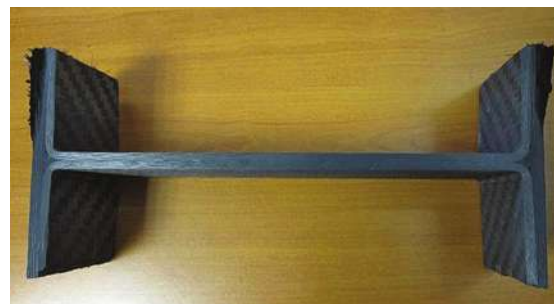
Researchers found that the last-filled zones corresponded with good precision to dry spots identified on the actual part (shown).
