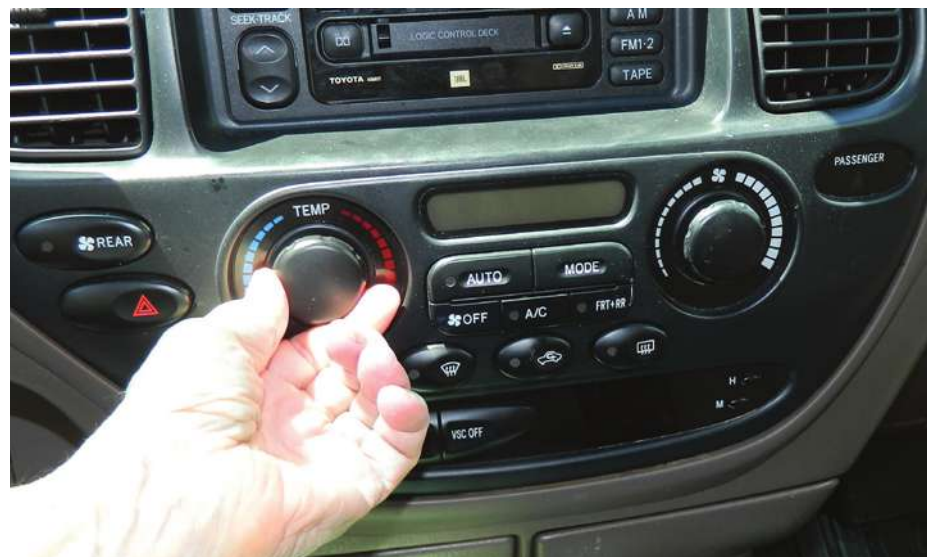
The AC17 test for manual temperature control system starts with full-cold and high-blower settings, then switches to midpoints at first idle of the SCO3 test.
