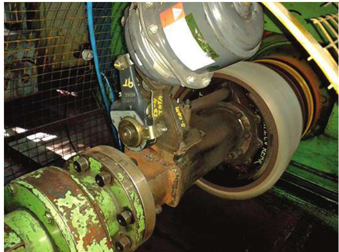
Dynamometer testing of bimetal brake drum.
