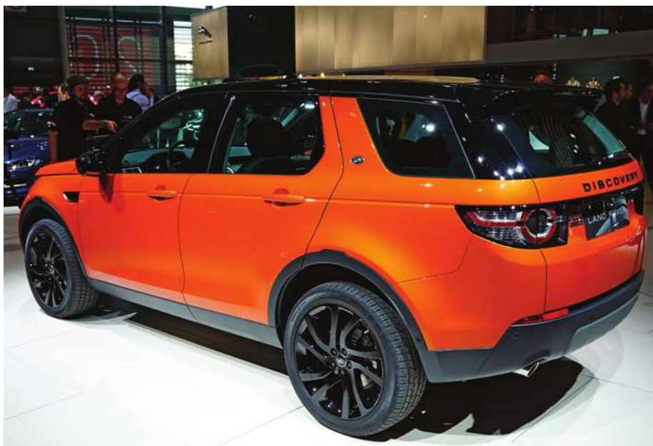
Hood, roof, and tailgate are manufactured in aluminum to aid weight reduction
