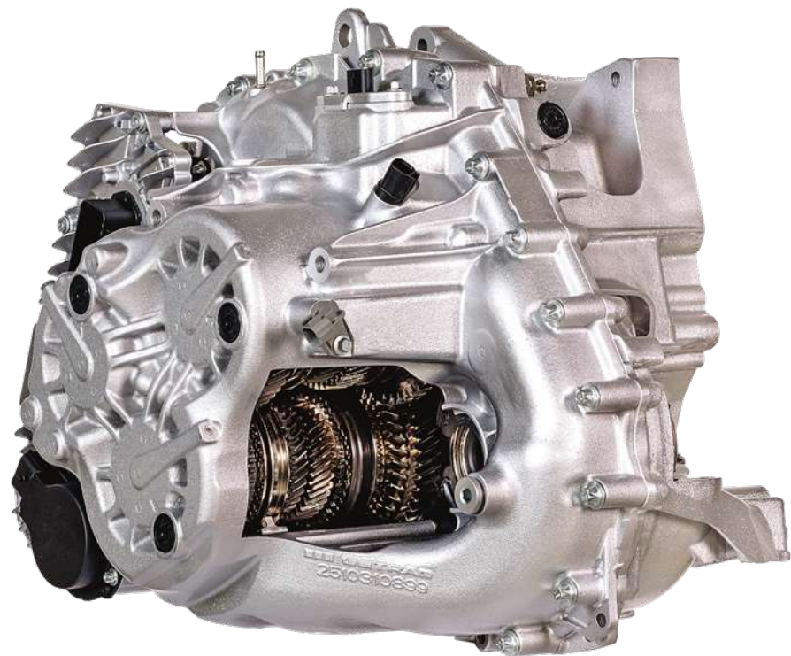
Renault is equipping its conventional vehicles with a new seven-gear dual-clutch transmission, developed by Getrag.
