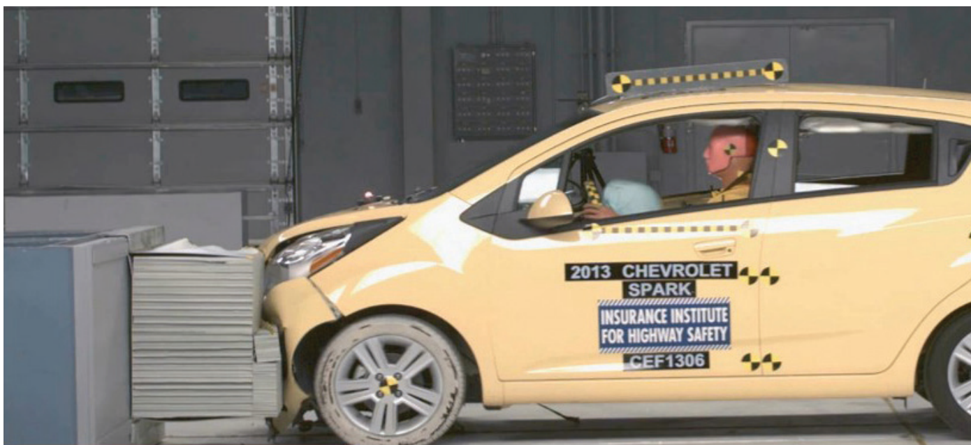
The 2014 Chevrolet Spark was the only vehicle in the Insurance Institute for Highway Safety minicar segment to earn a Top Safety Pick rating in 2014 model year testing (2013 model shown). Spark's safety structure makes extensive use of high-strength and ultra-high-strength steels and includes 10 standard airbags.
