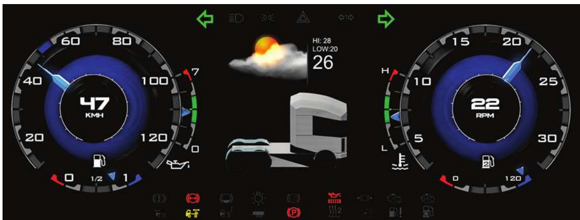
Crucial driver information is displayed within a 20° field of view and with photorealistic 3D graphics.
