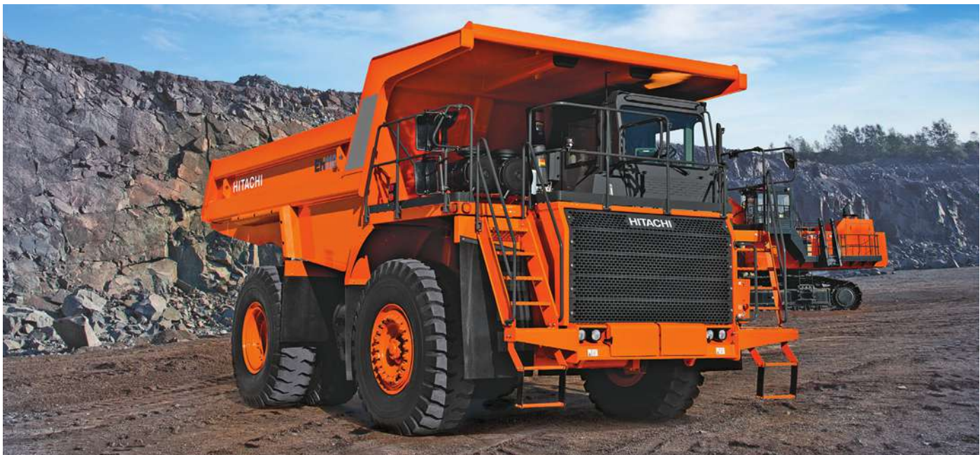
The latest version of the Hitachi's rigid frame dump truck, the EH1100-5, includes improvements to the operator environment, increased machine serviceability, increased payload, and more remote monitoring capability.
