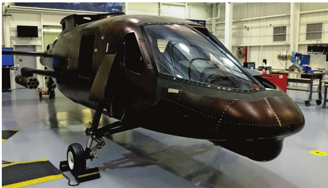
Sikorsky turned on electrical power to the S-97 in May. At that point, the aircraft was about halfway through the assembly process.
