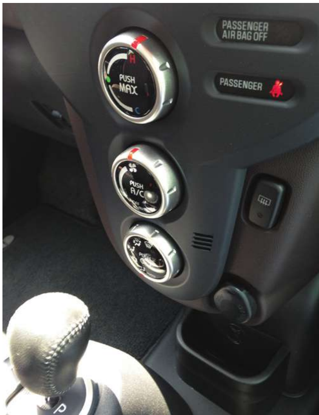
The Mitsubishi i-MiEV climate control panel is fully manual, and a study shows a large difference in EV range for normal vs. maximum settings.
