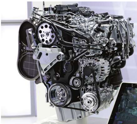
The most powerful of the diesels for the new Passat produces 176 kW (236 hp) and 500 N·m (369 lb-ft).
