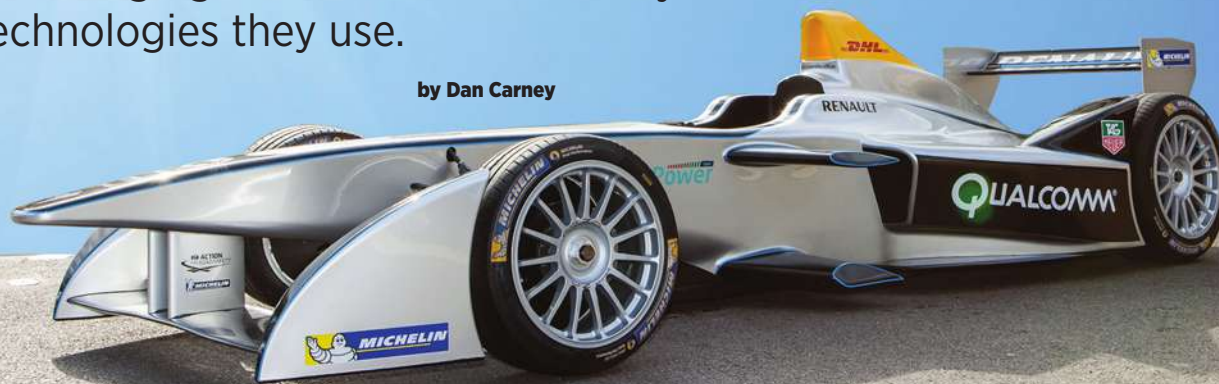
The Spark-Renault SRT_01E, with its aerodynamic shrouds ahead of its wheels, strongly resembles the current Indycar, which is also built by Dallara.
