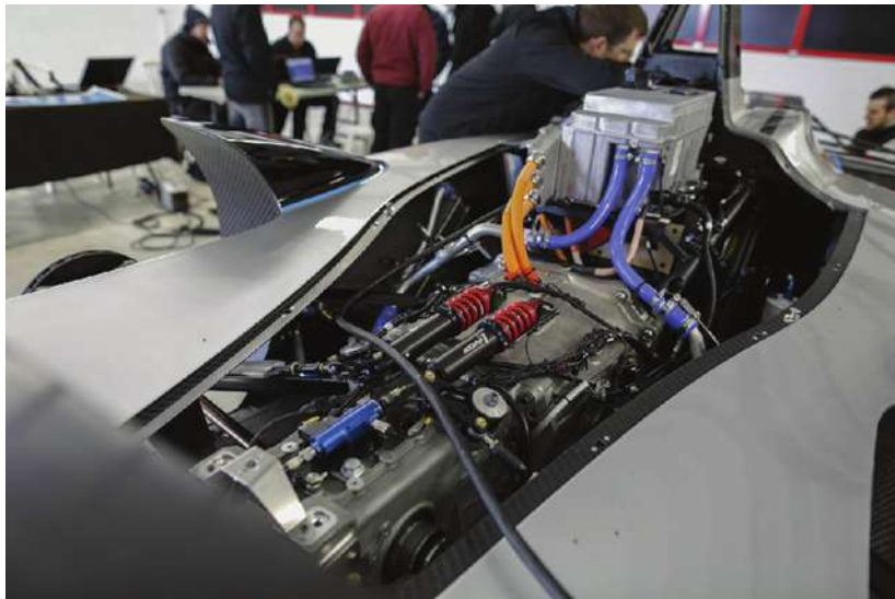
With its controller atop the electric motor, the McLaren powertrain resembles that of a conventional formula car with an inline engine.
