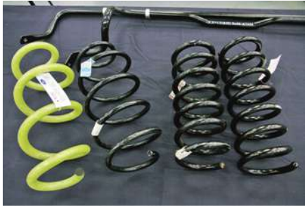
Composite (left) and hollow steel coil springs are featured on the Ford lightweight concept vehicle.
