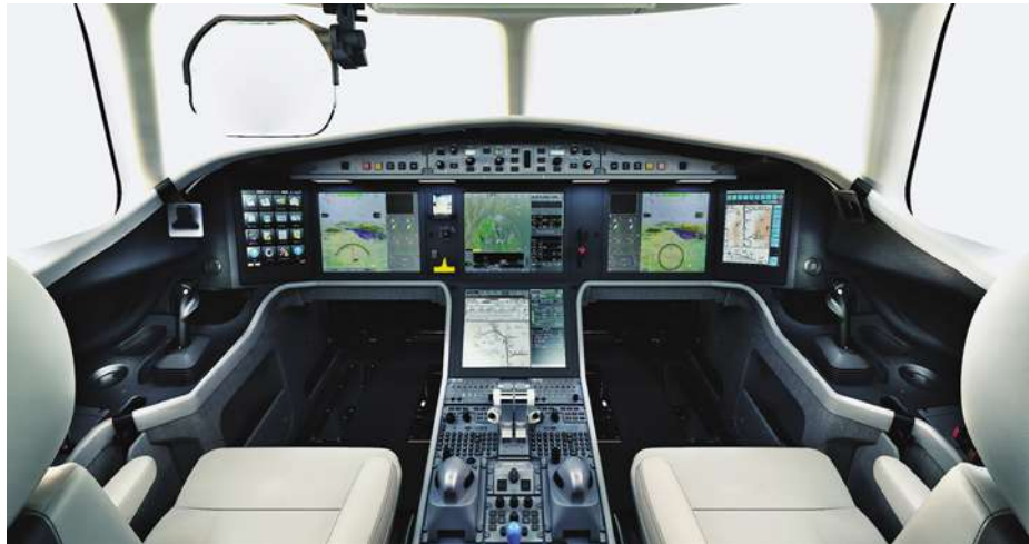
Dassault Aviation's Falcon 5X's EASy flight deck features 32% more window area, dual HUD capability with SVS and EVS, and an EFB that is integrated into the front panel.
