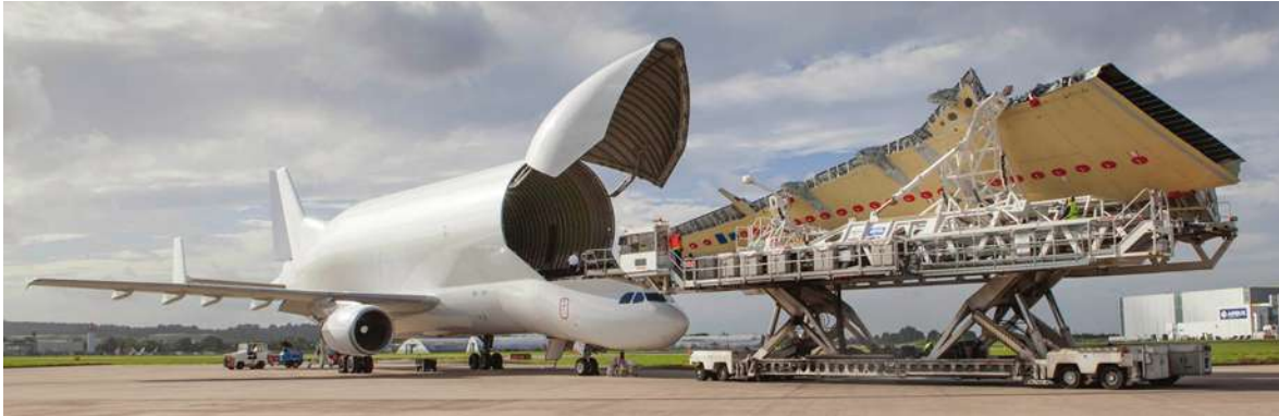
An Airbus Beluga loading an A330 wing at Broughton, U.K., for delivery to Toulouse, France for final assembly.
