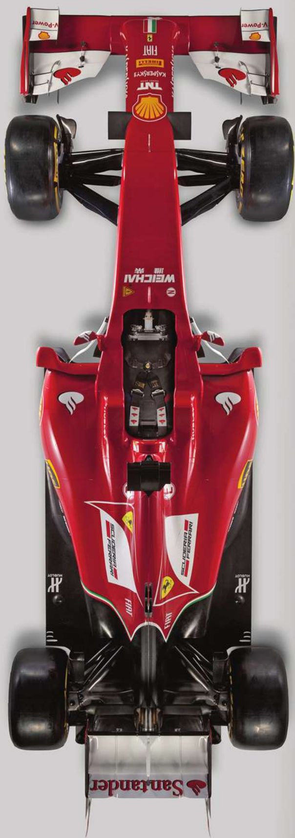
The Ferrari F14T illustrates how the 15-cm (5.9-in) narrower front wing leaves the front wheels more directly exposed to the airflow.
