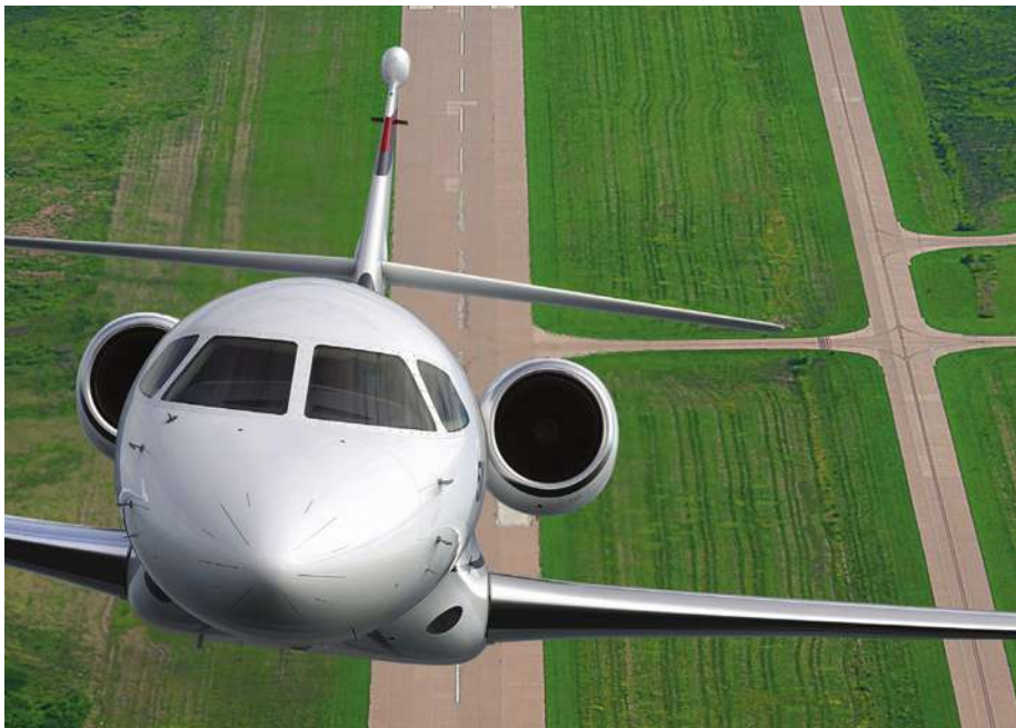
The Falcon 5X is the first aircraft in the business sector to use flaperons—active high-speed deflection control surfaces that can act as flaps or ailerons.
