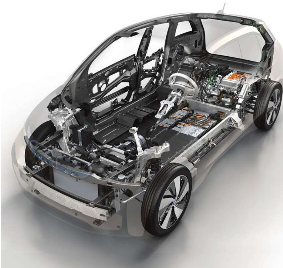
Adhesives are used extensively in the BMW i3, which features a carbon-fiber-reinforced-plastic passenger cell and aluminum structures. Dow Automotive, for example, optimized its Betaforce structural adhesives for the program. (BMW)
