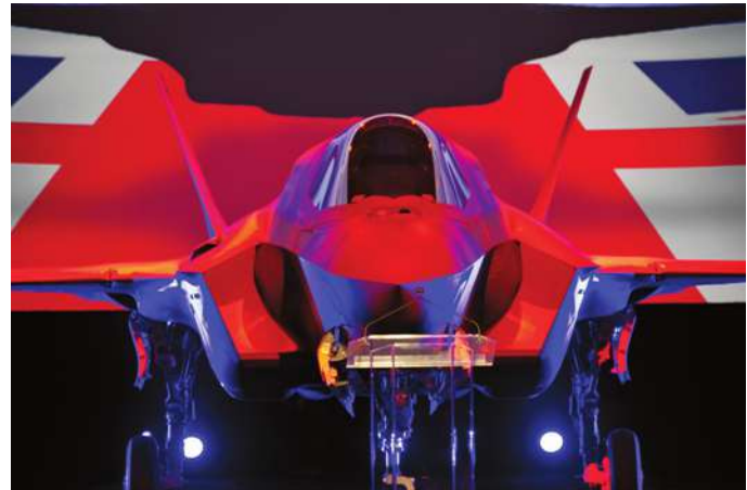
The U.K. aerospace industry has a major share in the F-35 program, producing rear fuselage and fin assemblies and the ejector seats and providing the Rolls-Royce lift fan that gives the F-35B model its vertical takeoff and landing capability. (MOD)
