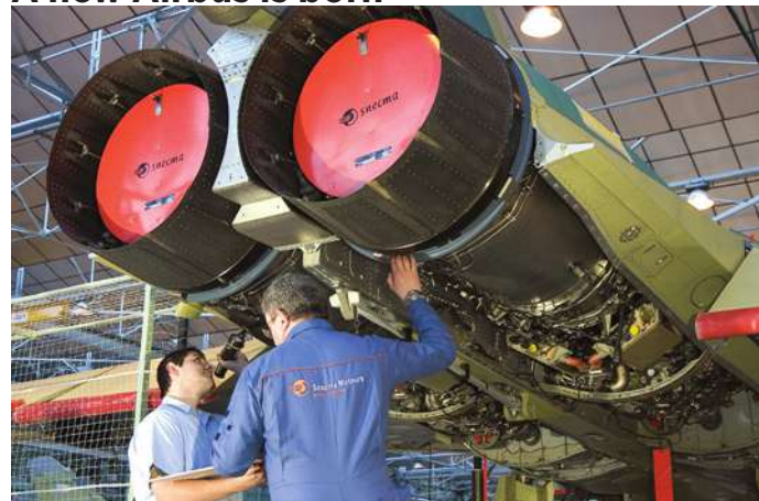
Snecma's M88 engines power the Rafale, and the core of the engine has been adopted for the A400M's turboprop engine that will be developed in a new open rotor prototype program.
