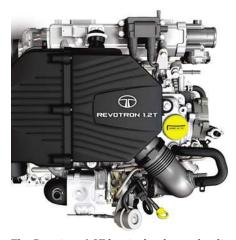
The Revotron 1.2T is a turbocharged unit delivering 140 N·m (103 lb·ft) from 1750– 3500 rpm and 85 PS (84 hp) maximum power at 5000 rpm.
