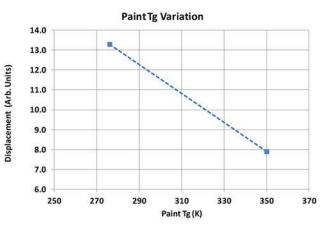
Surface displacement of paint dependence on glass transition temperature, t<sub>9</sub>. For illustrative purposes, note that only the temperature dependence of the paint CTE was modeled.
