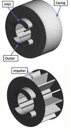
The same mesh was used for both the MRF and the sliding mesh calculations to achieve mesh consistency between the two models for relative comparison and assessment.
