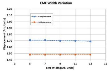
Variation of the EMF width by a factor of 2.6 for both Al and Cu. For this parameter set, the displacement remains essentially constant, but is significantly greater for Al than Cu.
