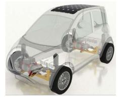
The EU's P-MOB microcar has a twomotor powertrain with independent batteries.
