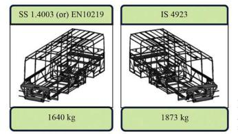
Difference in cumulative structure weight between SS and conventional steel.
