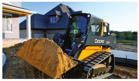
Deere says it is offering all major control patterns on the new models to meet customers' specific needs, including traditional hand and foot controls, hand-only controls, or low-effort, electrohydraulic joystick controls in both the ISO and "H" patterns.
