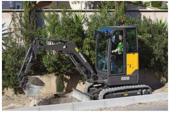
The access area into the cab is large enough that operators can get in and out easily without bumping controls, and a flat, uncluttered floor offers ample foot space.
