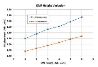
Variation of the EMF height by a factor of 2.7 for both Al and Cu. For this parameter set, the displacement increases with metal height and also is significantly greater for Al than Cu.
