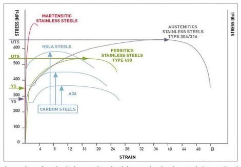
Comparison of mechanical properties of stainless steel and carbon steel. (International Stainless Steel Forum)
