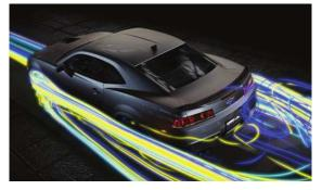
The Z/28 features rocker moldings and unique wheelhouse extensions that help push air past the tires. Deflectors at the bottom-front corners of the front wheel flares take the place of a conventional air dam.
