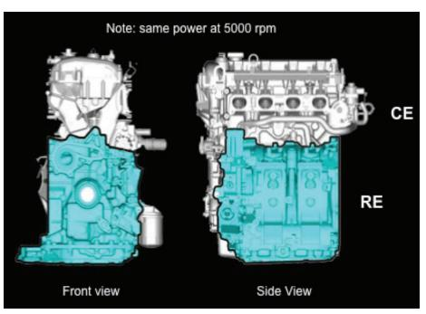
Mazda illustrates how its compact 330-cc single-rotor rotary engine (shaded blue here) compares in size to a piston engine of equivalent power.
