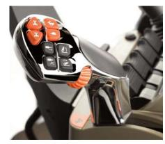
An improved Multicontroller provides for simplified operation and optimum workplace ergonomics. It is fitted with backlighted operating keys allowing for easier and safer operation in the dark.
