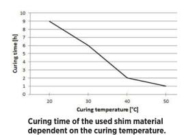
reduced; a decreased temperature leads to longer curing times. Especially during winter (with shop-floor temperatures less than 20°C), this could lead to curing times of up to 16 h.
