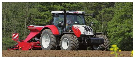
With Steyr S-Tech, the engine and CVT, electronic hitch control, PTO, four-wheel drive, and differential lock, as well as additional controls and S-Guide auto steering, are all interlinked.
