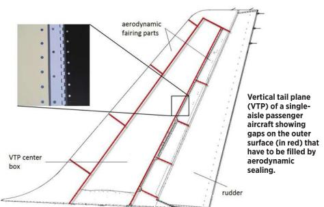
Researchers from **Airbus Operations** GmbH and **Marcotodo** GmbH describe two applications of heated air technology for the accelerated curing of resin-based shim and sealant materials. The first example is the aerodynamic sealing of a VTP; curing time of the aerodynamic sealant can be reduced by 8 to 10 h using the newly developed heated air namic sealing, has to be performed to smooth the surface.
