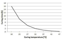
Curing time of the used sealant material dependent on the curing temperature.
