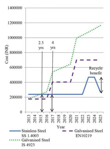
LCC trend over the expected life of a bus. The initial cost difference of stainless steel is bought back in 2.3 years compared to conventional structural steel and in 4 years compared to galvanized steel of equivalent strength.
