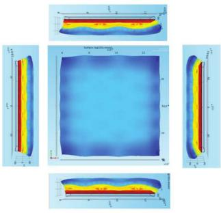
Von-Mises stress patterns due to thermal air to ground heating cycle. EMF mesh bleed-through is evident in the central portion of the figure and relatively large displacement variations are observed above the metal and voids. Note that the displacements have been magnified for illustrative purposes.
