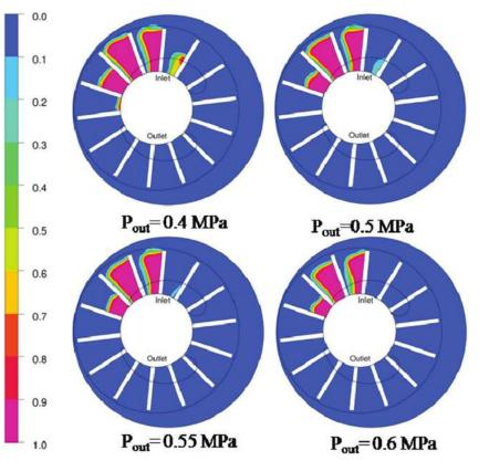
The vapor fraction distribution predicted by the MRF approach indicated an unrealistic unphysical location of cavitation. As can be clearly seen, the MRF model predicted that the cavitation occurs near the inlet port, which is not possible.
