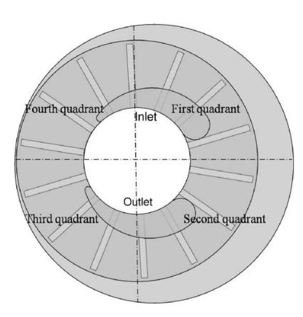
The liquid ring pump configuration that was studied consisted of a single-stage impeller with 14 blades arranged in an equispaced manner circumferentially.
