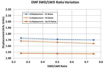
EMF displacement dependence on metal mesh SWD/LWD ratio for Al and Cu. (FG = fiberglass)
