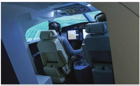
The Falcon Simulation Bench comprises a cockpit mock-up coupled to a real-time simulator and a panoramic external visualization system depicting the artificial flight environment. It allows pilots to test all phases of flight, from takeoff to landing, and to fine-tune and validate control laws before the maiden flight of the aircraft.
