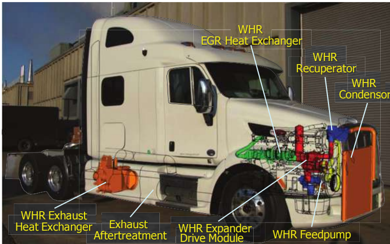
Installation of the WHR system in a Class 8 tractor.
