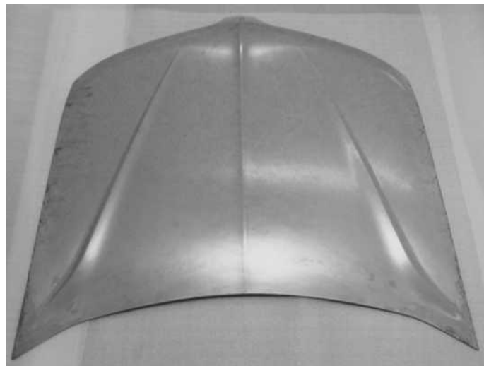
Low-density SMC outer panel of CSP's two-part prototype hood provides robust exterior with good surface appearance.
