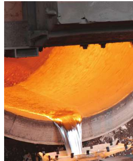
At its Issoire recycling casthouse, Constellium has demonstrated the recyclability of A300 wings and cockpit parts with a recovery yield of over 90%, resulting in new aluminum ready for use in future aircraft.
