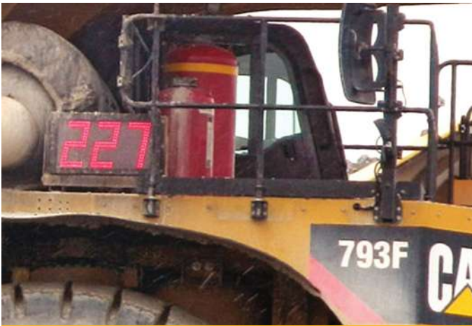
Measuring the weight of a payload helps Caterpillar improve safety of heavy mining trucks.
