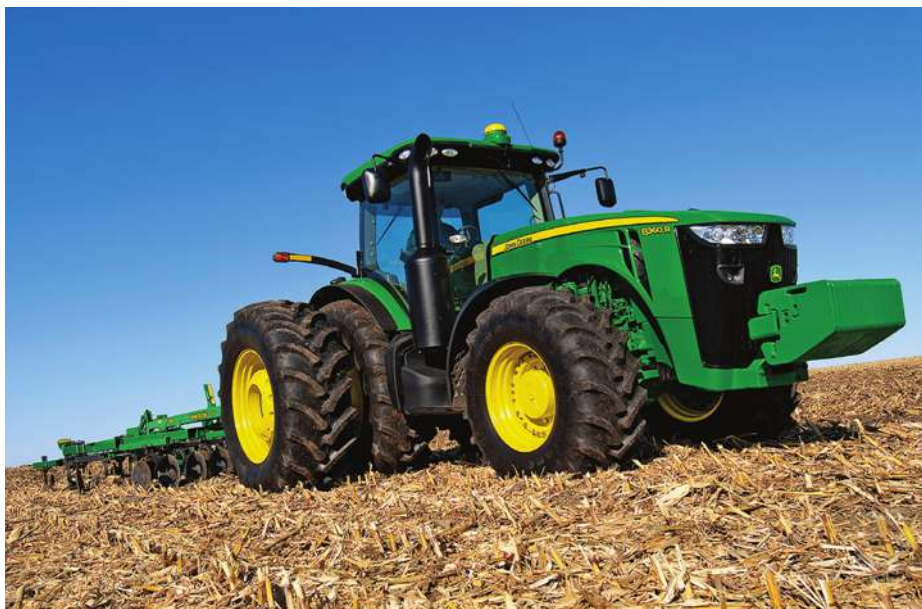
Deere engineers increased the engine power ratings of all the new 8R models and boosted the maximum hydraulic flow capacity by 41% to 85 gal/min.
