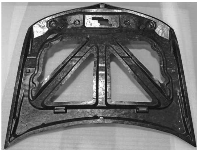
Carbon-fiber-reinforced SMC hood inner structure adds strength to CSP's two-part composite hood prototype.
