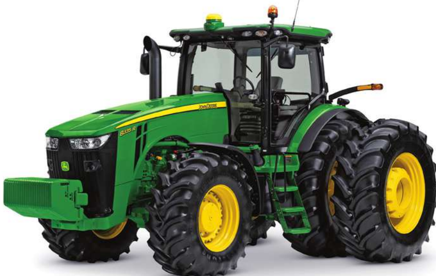
The new CommandView III Cab features laminated glass, a strategically placed insulation barrier, and an optional carpet floor mat to reduce noise and vibrations.
