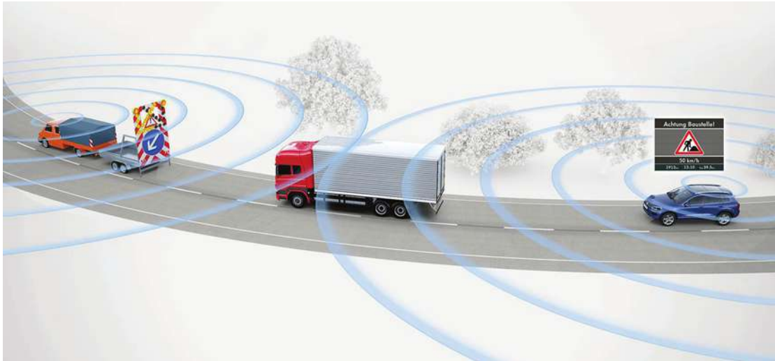
“Seeing” around the corner: VW’s Car2X communication system promises significant support for driver safety when approaching road work.
