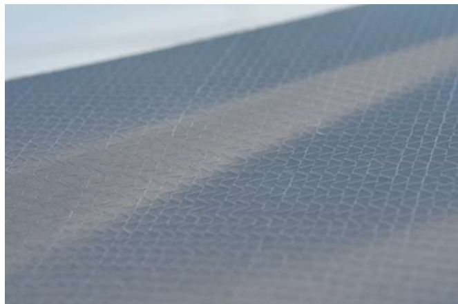
Close-up of Ford's experimental CFRP hood—a sandwich construction—shows the surface before exterior finishing.
