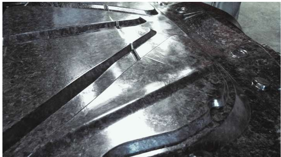
Close-up of CSP's prototype inner hood member shows the 1-in (25-mm) chopped carbon fiber used as the reinforcement.
