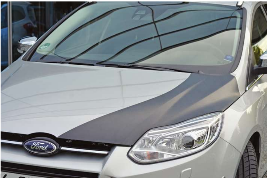
Ford is developing a prototype carbon-fiber hood (partially exposed) for its Focus compact that weighs 50% less than standard steel.
