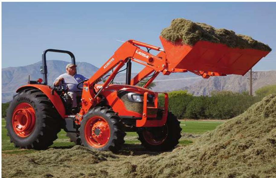
The LA1154 front loader is also equipped with a series valve with regenerative function, which allows simultaneous lift and dump or rollback and raising of the bucket.
