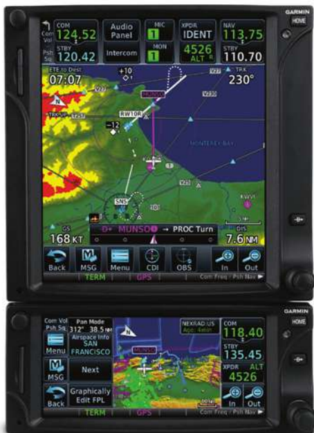
Pilots can adjust views by touching Garmin's interactive display panels.
