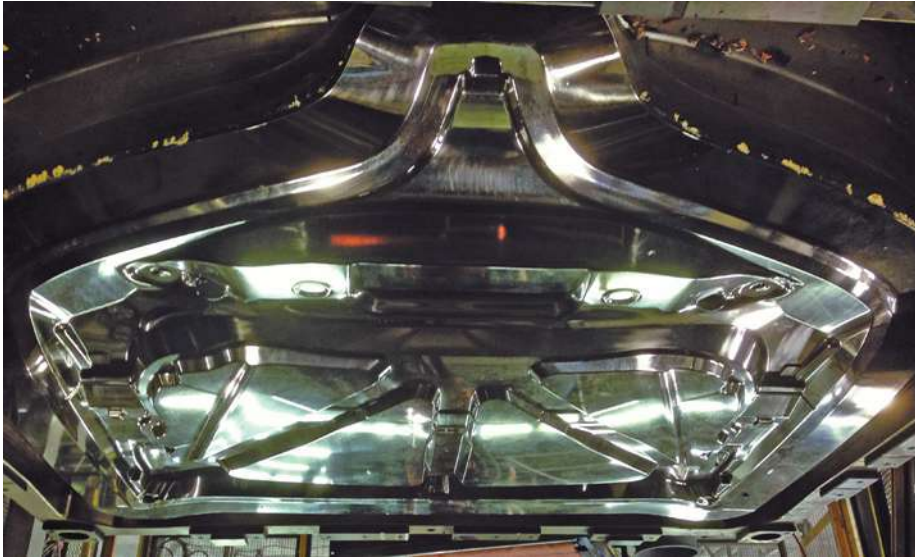
CSP engineers created an experimental tool to form the inner CFRP member of its lightweight hood prototype.
